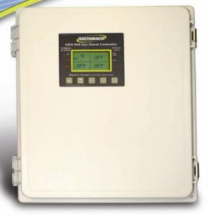
Bacharach's GDA-400 four channel controller is designed to provide simultaneous display and alarm functions for up to four monitors with 4-20 mA inputs. A graphic LCD displays monitored data as gas type and concentration, bar graphs and 30 minute trends. Three adjustable alarm levels are provided per channel. Relay outputs allow control of audible and visual alarms, strobes, horns and other alarm events.
