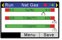
Using color-coded arrows, Tune-Rite <sup>™</sup> shows which readings are in range (green), unstable (yellow) or out of range (red).
